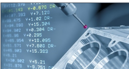
Measurement inside the machine, part still clamped.
