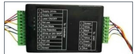
Interface unit and terminal connections.
