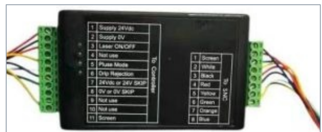
Interface unit and terminal connections.
