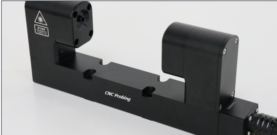
CNC Probing non-contact laser tool setter. Transmitter and receiver face each other; when the tool enters the beam path the system produces a trigger signal.
