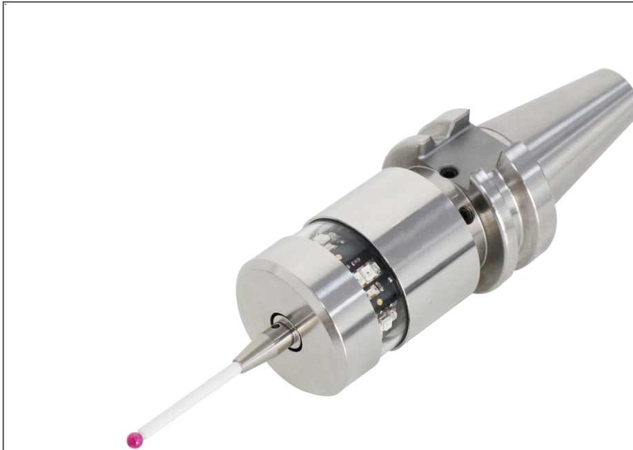
CNC Probing infrared measuring probe. It mounts in the spindle taper; transmission is 360 degrees around the probe axis.
